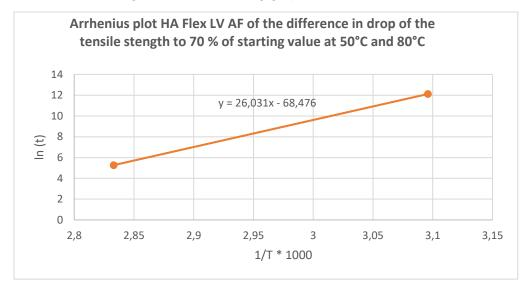
In this way it can be calculated how long it would take at  $20^{\circ}$ C for the tensile strength of HA Flex LV AF to drop to 70 % of the starting value :
